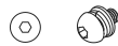
M6 x 15 mm Machine Screw with Lock Washer and Flat Washer x 24
