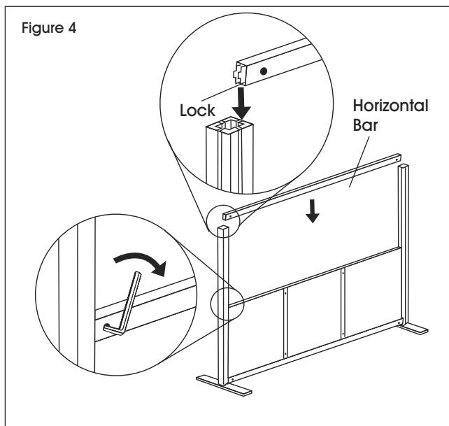
6. Insert horizontal bar between posts and slide onto top row of panels. Tighten locks using Allen wrench. (See Figure 6)
