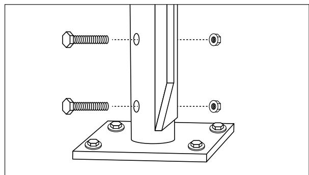
1. Using pre-drilled holes in base of mount as templates, mark the location for each hole on the concrete surface.
