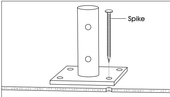
1. Using pre-drilled holes in base of mount as templates, mark the location of each hole on the asphalt surface.
