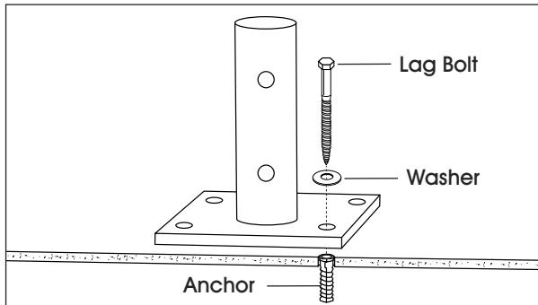
3. Redrill holes with a 3/4" masonry bit to the depth required for the anchors.
