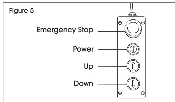
8. Run the table up and down several times to remove any air that may have been trapped in the hydraulic system during shipment.
