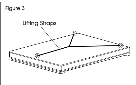
4. Using a forklift or suitable lifting device, raise the lift table using the lifting straps, remove pallet from beneath lift table and set lift table down into desired location. Once set, remove lifting lugs from the lift table.
