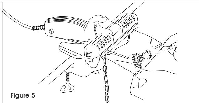
3. Take pressure off the foot pedal to release the sealing jaw and remove the bag. (See Figure 7)
