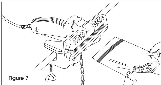
4. If not using the foot pedal, insert bag into the sealer and squeeze the handle of the unit together. Hold to seal the bag. (See Figure 8)
