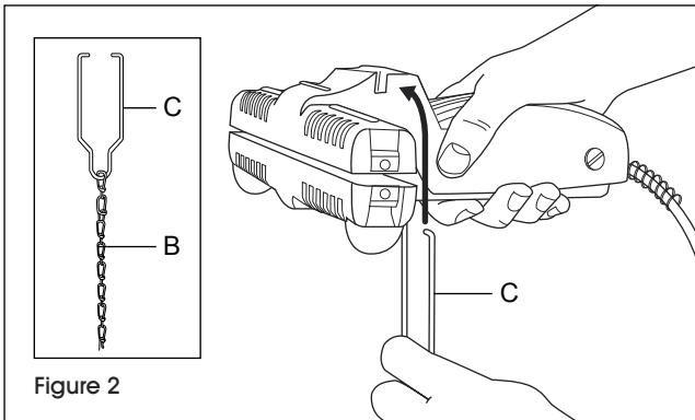
3. Rest the sealer on the clamp brackets. Attach the other end of the chain to the "S" hook on the foot pedal (D). (See Figure 3)
