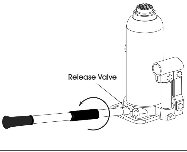
2. Move handle into handle socket and rapidly pump the handle 6-8 times. Leave handle in down position to expose oil fill plug. (See Figure 2)
