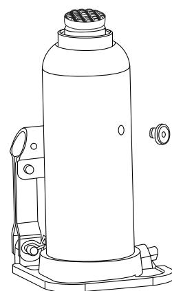
3. Fill the oil case until oil level is just beneath lower rim of oil fill hole. (See Figure 10)
