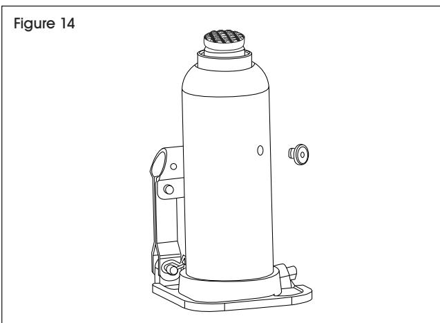
4. Turn jack on its side so old oil will drain from oil fill hole. (See Figure 15)
