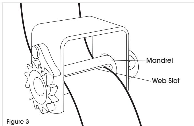
3. Tighten the winch strap using a winch bar to the appropriate tension. The winch bar should be inserted through both sides of the mandrel cap on the winch. (See Figure 4)
