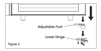
Remove the hinge sleeve from the bottom left side
