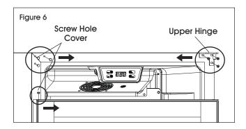
Install the upper hinge on the upper left side of the cabinet. Install the screw hole covers on the upper right side of the cabinet. Install the door onto the cabinet. Install the adjustable foot and lower hinge on the lower left side of the cabinet. (See Figure 7)
