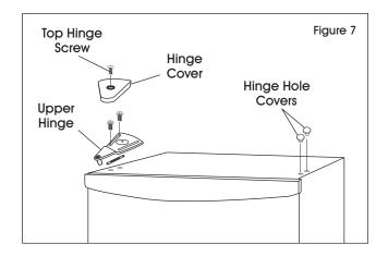
5. Install the hinge cover over the hinge and install the hinge hole covers in the screw holes on the top right side of cabinet. (See Figure 7)
