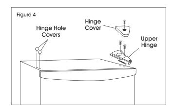
2. Remove the hinge hole cover from the top left side of the door and install it in the hinge hole on the top right side of the door. (See Figure 5)
