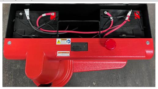
Prior to leaving the factory, two battery leads in the battery section have been disconnected. To provide power to the machine, these leads will need to be reconnected.
