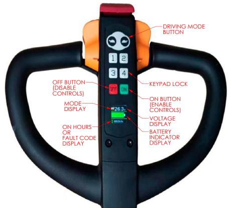
CONTROLS OPERATOR SIDE HANDLE ARM RAISED
