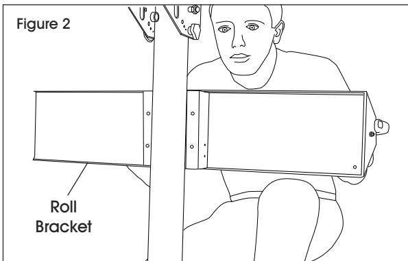
2. Place small roll bracket plate on opposite side of stand. Align four screw holes on roll bracket and small roll bracket plate. Screw tightly to secure roll bracket on stand using a drill or Phillips screwdriver. (See Figure 3)
