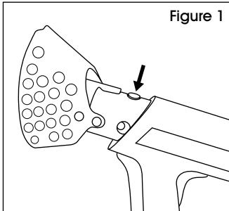
3. Assemble the remainder of the tool into the open end of the extension tube. Confirm it is locked in place by ensuring the #31 button protrudes from the extension tube. (See Figure 3)
