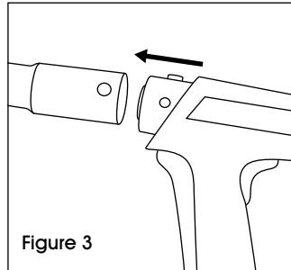
2. Attach combustor to end of the extension and confirm it is locked in place. The #31 button should protrude from the hole in the combustor when locked. (See Figure 2)
