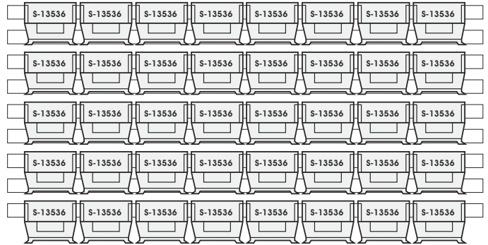
4" tall / 4" wide bins: (including S-13536) Fit 8 per row, 40 on each side, 80 bins total
