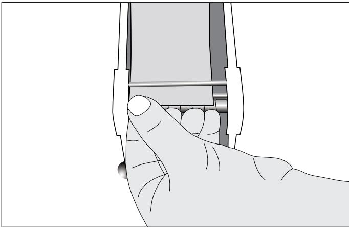
3. Feed liner between second bar and coiled third bar.
