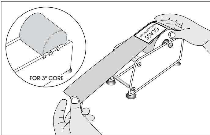
2. Feed liner under the first bar and over the second bar.
