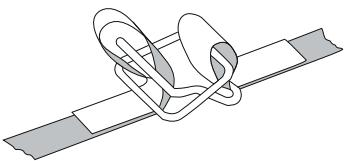
2. Put strap and buckle around package and manually tighten the strap. (See Figure 2)
