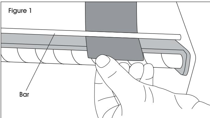
2. Insert the liner between the plastic plate and coil. (See Figure 2)
