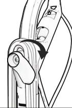
5. On models with cleaning attachments, place the wand into the lower retainer. Ensure the suction valve is set to the floor cleaning position. Secure the wand into the wand clip.
