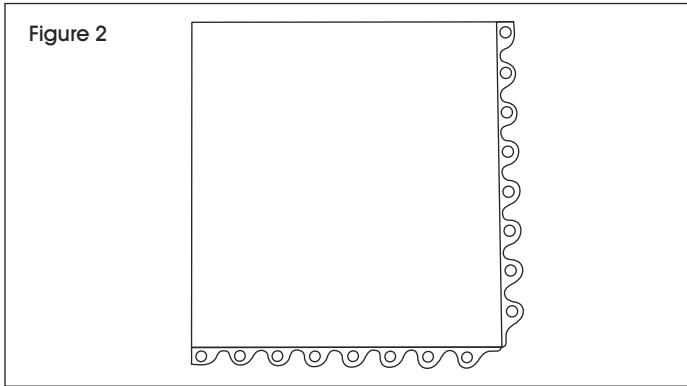
2. Place second tile adjacent to first with sockets of second tile facing pins of first tile. Snap pins into sockets. Continue to install mat tiles one row at a time, snapping pins into sockets. (See Figure 3)
