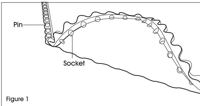
1. Place one mat tile in corner, flush against wall or in desired location.
