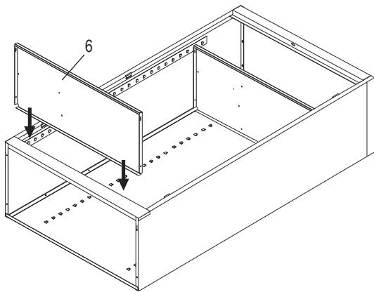
7. Insert partition (7) into the cabinet. Align the two top and two bottom holes in the partition with the holes in the top of shelf and bottom of cabinet. Attach with bolts and nuts. (See Figure 6)
