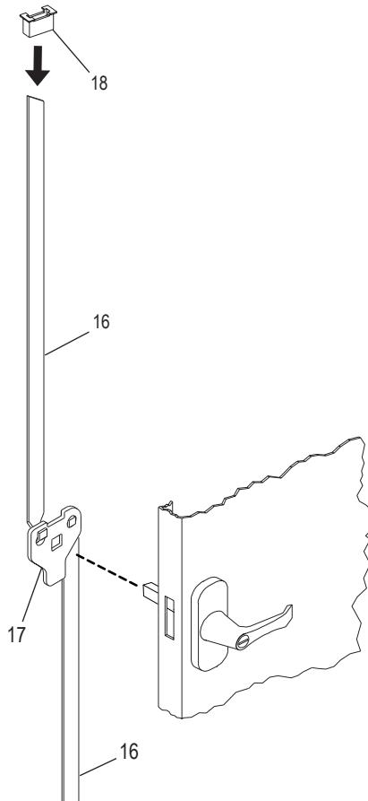
1. Place the door handle (15) on the right hand door and fasten with two slotted bolts and lockwashers. (See Figure 10)
