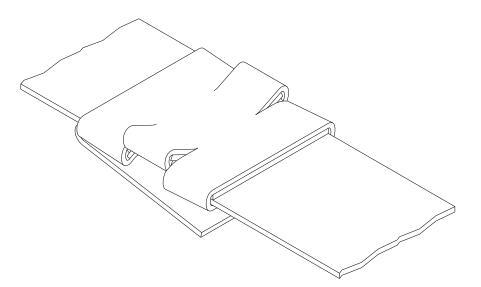
Sharp edged or misformed joints which do not appear as shown have to be taken away from the load immediately. The tensile strength of these joints is insufficient and they could cause serious injury. Having faulty joints proceed as follows:
