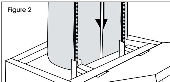
3. Push down and forward (keeping the cartridge at a 90° angle), ensuring all blue clips enter the track. Use both hands if necessary. (See Figure 3)
