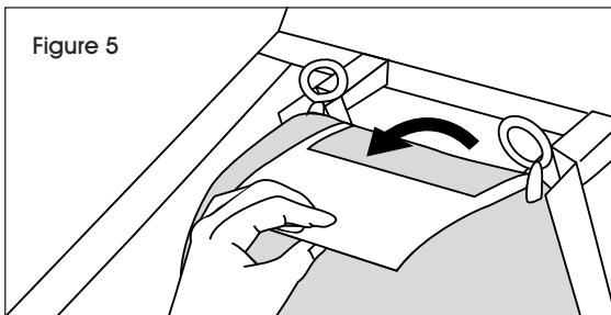
5. Place one hand on top of cartridge. While holding down the shoe covers, remove the orange tabs, one at a time. (See Figure 6)
