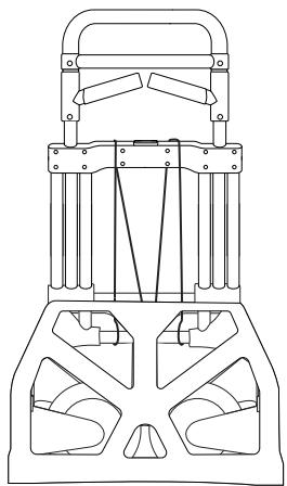
3. Tilt truck towards you with wheels slightly lifted off ground. Press down on nose plate to extend wheels. (See Figure 3)
