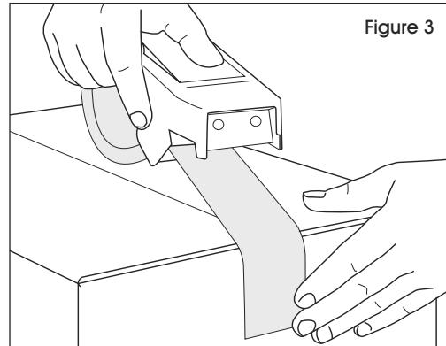
2. Pull dispenser across box top, over the center seam. Apply hand pressure on brake to provide tension on tape to obtain tight seal. Press tape down with opposite hand. (See Figure 4)
