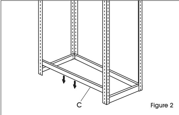
2. Connect the two upright post assemblies by inserting front/back supports (C) at the bottom of the upright posts. (See Figure 2)
