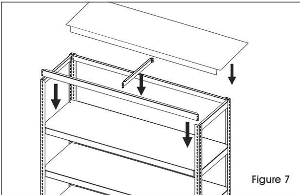
7. Attach remaining front/back support and shelf support. Lay the last steel shelf on the shelf supports. (See Figure 7)
