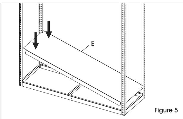
5. Lay the bottom steel shelf (E) on the shelf support so that the front and back edges overlap the front/back supports. (See Figure 5)
