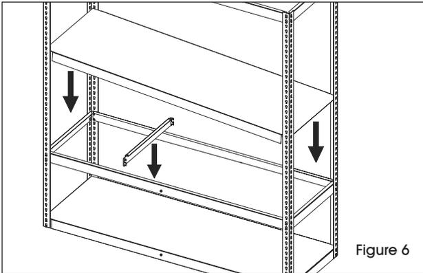
6. Attach front/back supports at the desired next level. Attach shelf support, then lay the steel shelf on the shelf support. (See Figure 6)
