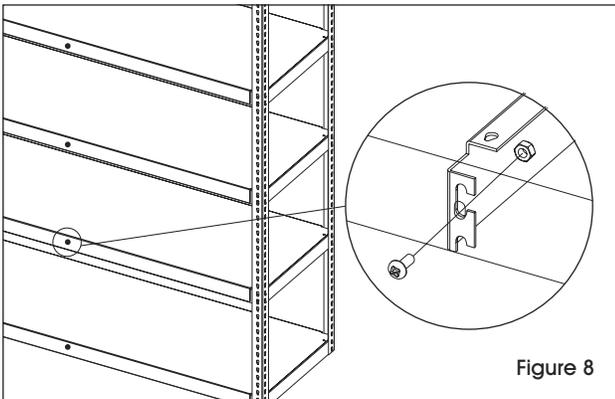
8. Once the shelves are in place, if additional stability is desired, secure the shelves with nuts and bolts (F). Fully tighten. (See Figure 8)
