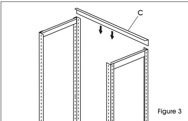
3. Connect the top of the two upright post assemblies by inserting one front/back support (C). (See Figure 3)
