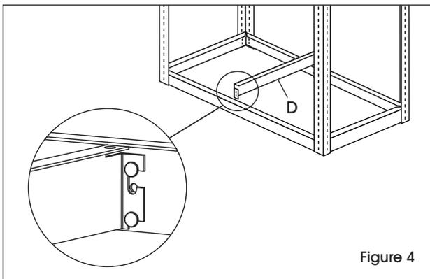
4. Attach shelf support (D) at bottom level by placing the keyhole slots (on shelf support) over the rivets (on front/back support) and tapping them into place. (See Figure 4)
