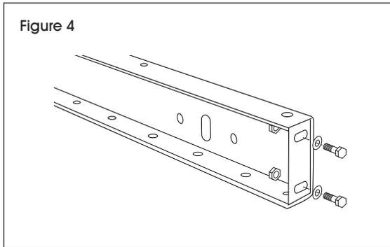
2. Fasten the bolts through the ends of both conveyor frames, using the same holes that they arrived in. (See Figure 5)
