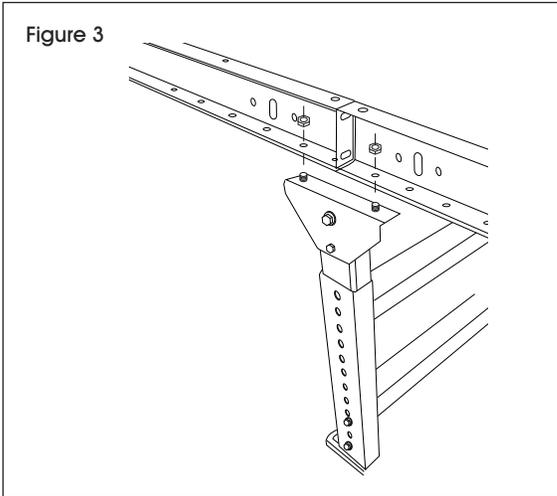
**NOTE:** Each conveyor frame includes mounting holes for an optional center leg support. Adding a third support increases weight capacity.
