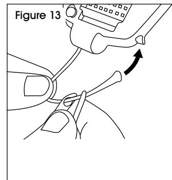
3. Close the locking mechanism and apply padlock.
