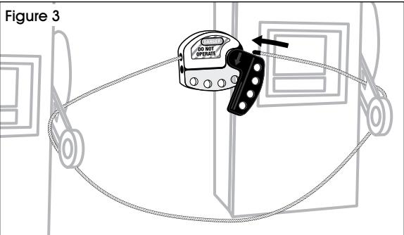
4. Insert the end of the cable into the lockout device. (See Figure 4)
