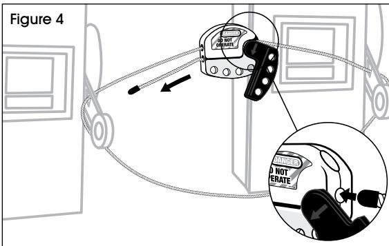
5. Close lockout handle and pull the cable through until it is taut. Insert the padlock and secure. (See Figure 5)
