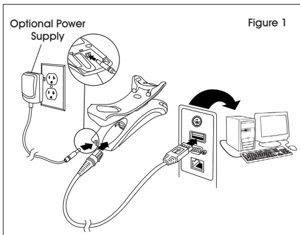
2. Ensure the cable is secured in the wireways in the bottom of the base and that the base sits flat on a horizontal surface. The scanner will beep.
