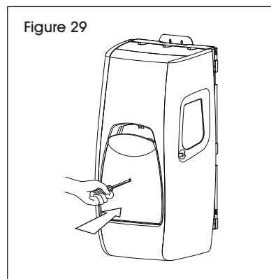
4. While button is pressed in, gently pull door open (there should be no resistance). (See Figure 30)
