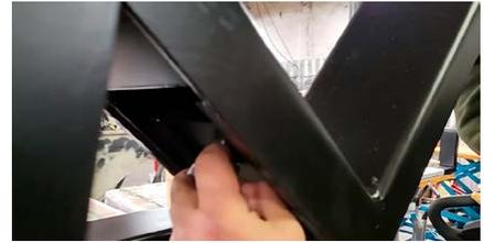
5. Turn the adjustment knob clockwise to reduce the height of the end of the fork tip from the floor or counterclockwise to increase the height of the end of the fork from the floor.
