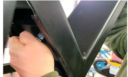
6. Tighten jam nut by turning clockwise until hand tight. Then turn adjustment knob clockwise to essentially further tighten the jam nut.
