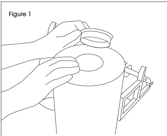
3. Place roll on support tube into frame as shown.
