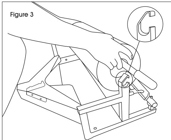
2. Insert support tube into core of roll.
