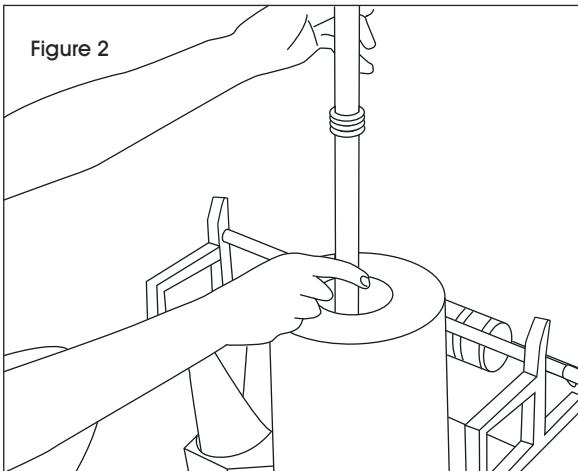
4. Feed paper under brake and then over PVC roller.
