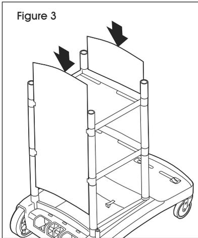
6. Slide two side panels into sides of cart as shown. (See Figure 3)
