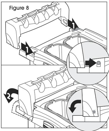
12. Slide tool grip into opposite side of handle and rotate down to lock into position. (See Figure 8)
