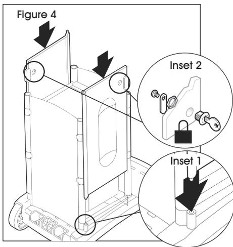
7. Slide door panels down two other sides of cart, ensuring that bottom aligns into holes correctly. (See Figure 4) (See Inset 1)
