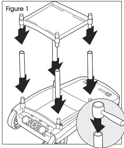
1. Place four long aluminum uprights onto pegs on base. Use rubber mallet to secure in place. (See Figure 1)
