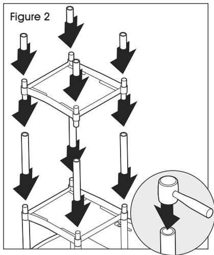
3. Place four long aluminum uprights onto pegs of first shelf. Use rubber mallet to secure in place. (See Figure 2)
