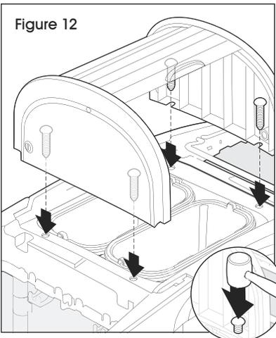
16. Place locking security hood on top of open shelf. Then insert bolts into four locations inside lid as shown. Use rubber mallet to set in place. (See Figure 12)
