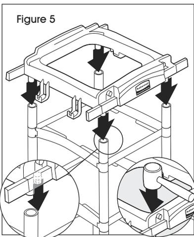
9. Place open top shelf onto short aluminum uprights. Use rubber mallet to secure in place. (See Figure 5)
