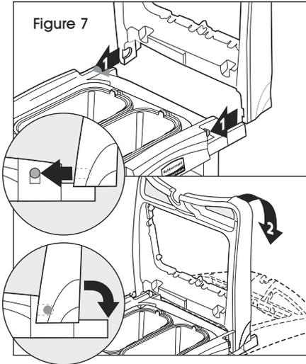
11. Slide handle onto open top shelf and rotate down to lock into position. (See Figure 7)
