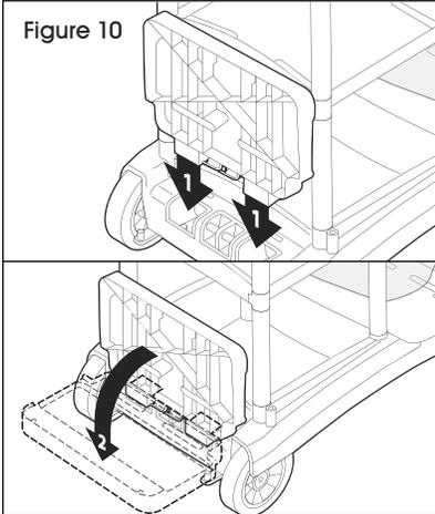
14. Snap mop bucket platform down into place and then lower platform into position. (See Figure 10)
