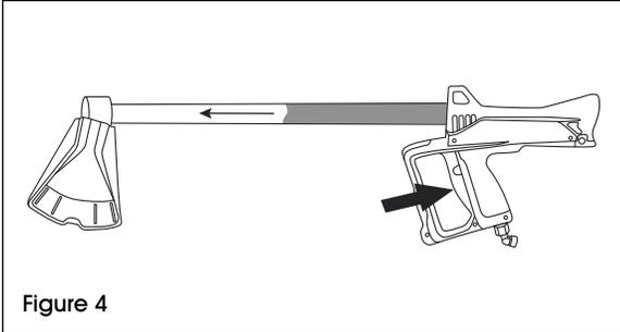
2. After allowed time, fully press down on the trigger to ignite heat gun. (See Figure 5)
