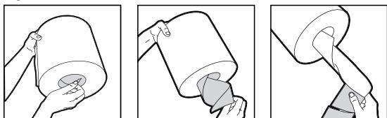
2. Pull toweling from the center of the roll and pinch the end of the toweling enough to slide into the dispensing cone. (See Figure 4)
