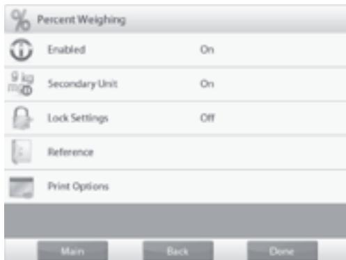
The balance can be configured to operate in various application modes. Touch **APPLICATIONS** to choose – or the top button in the application area.
