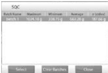
13. The Batch History screen shows the basic information – maximum, minimum, average (mean), and standard deviation – for all currently saved batches.
