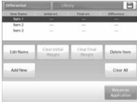
5. Enter the new name, then press **√**. The display returns to the previous screen with the new value highlighted momentarily.
