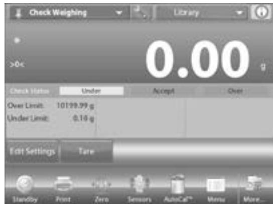
3. To use this mode, touch **EDIT SETTINGS** to set the target weight, and upper and lower tolerance values.
