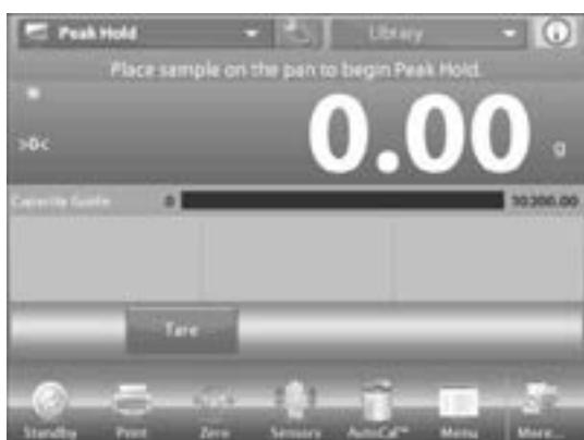
4. The highest stable weight reading is held until the weight is removed.
