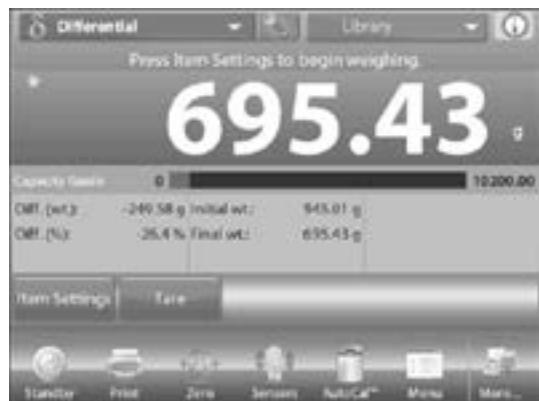
6. A message prompts for Item 1 to be placed on the pan again, then to press **ACCEPT** to establish final weight. After **ACCEPT** is pressed, the difference between initial and final weights appears in the Reference Fields.
