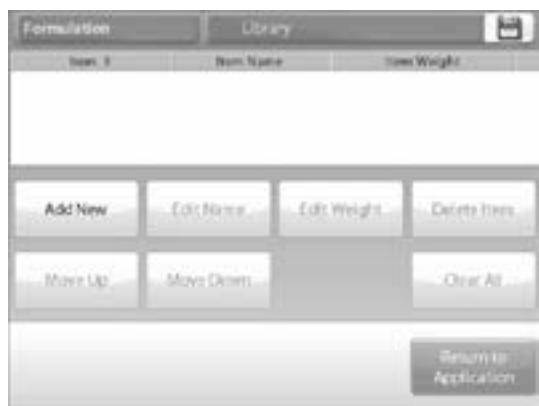
6. A new default component is added to the end of the formula (default name, weight). To change the default component name, press **EDIT NAME**. The alpha-numeric entry screen appears.
