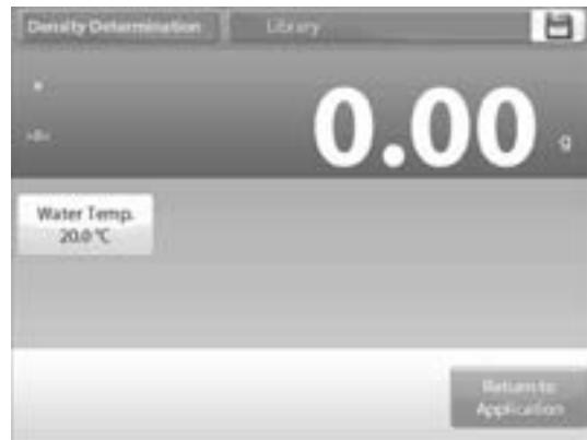
2. A numeric input window appears. Enter the actual water temperature, then press **DONE**.
