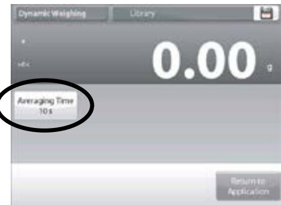
2. A numeric input window is displayed. Key in the desired Averaging Time, then press **DONE**.
