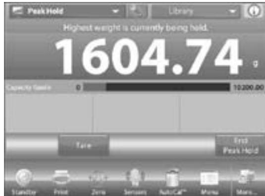
3. To release the reading, press **END PEAK HOLD**.
