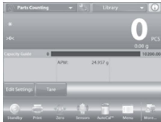
**NOTE:** Auto Optimization improves counting accuracy. It recalculates the piece weight automatically as parts are added. By default, auto optimization is set to "off".
