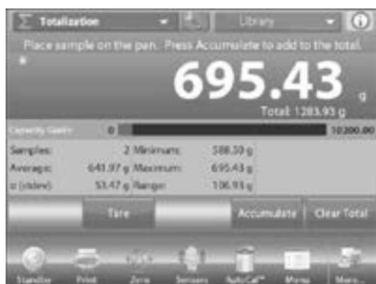
5. When stable, the new total is shown on the secondary display line.
