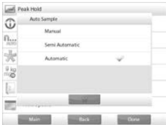
3. Place item on the pan. The capture process starts automatically.
