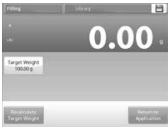
1. To adjust the Target Weight value directly, touch the **TARGET WEIGHT** button.
