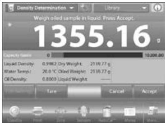
14. Once the necessary weights have been determined, the density of the sample is displayed in g/cm<sup>3</sup> (along with the weight in air, un-oiled and oiled, and weight in water) on the application screen.
