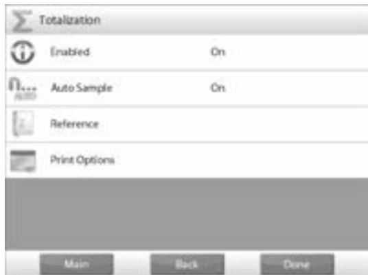
4. The weight of the item is automatically added, when stable, to the total. The new total is shown on the second display line.
