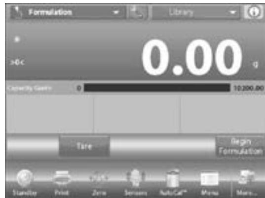
3. A prompt says place component 1 then press **ACCEPT**. The item weight is displayed on the main display line. Place the first ingredient on the pan (or in a tared container). Press **ACCEPT** to store the first component.
