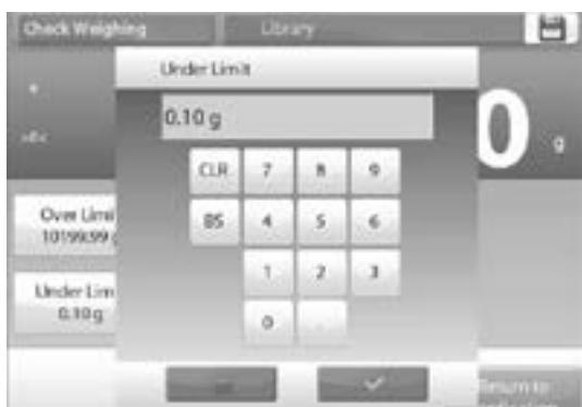
5. The display returns to the previous screen with the new value highlighted momentarily. To return to the check weighing home screen, touch **RETURN TO APPLICATION**.
