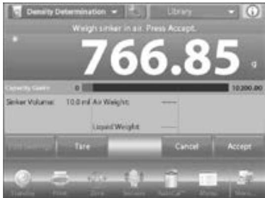
11. Once the necessary weights have been determined, the density of the liquid sample is displayed in g/cm<sup>3</sup> (along with the weight in air, weight in water) on the application screen.
