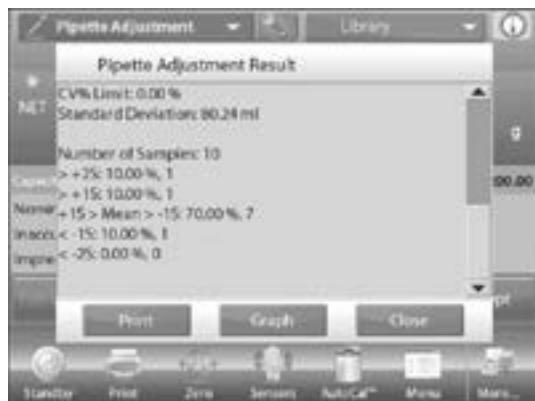
4. Press **GRAPH** to see results plotted. Press **RESULT** to return to the result screen. Press **CLOSE** to return to the pipette adjustment home screen.
