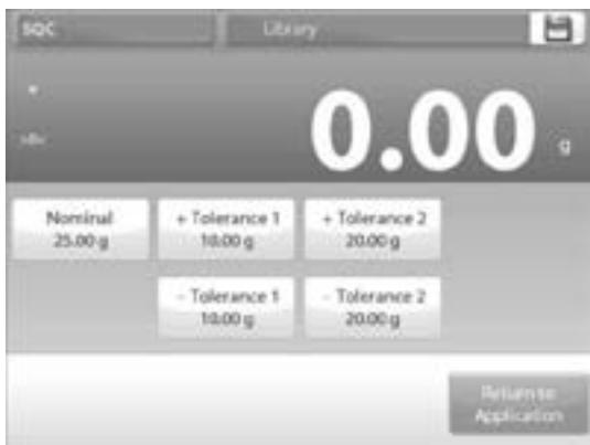
4. To adjust the Nominal Target weight value, touch the **NOMINAL** button. A numeric input window appears.
