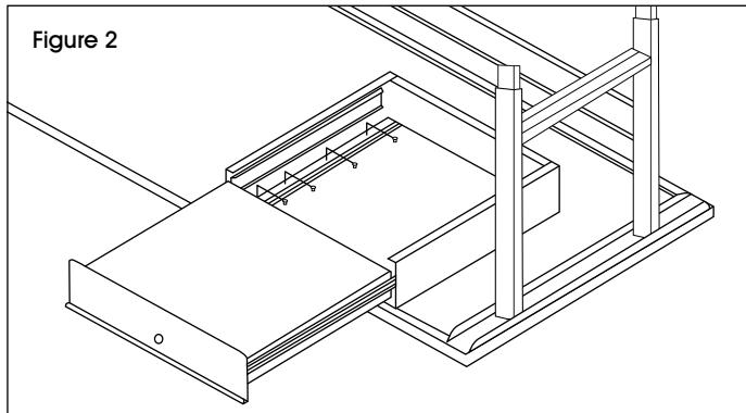
3. Close the drawer and turn packing table right side up. Cycle the drawer in and out a few times to check operation.
