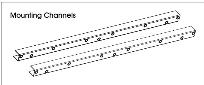
1. Turn the packing table over. On the underside of the table, slide mounting channels front to back into table flanges. When channels are aligned, mounting holes should be approximately 23½" apart. Secure each channel with two 1/4"-20 x 5/8" bolts. (See Figure 1)
