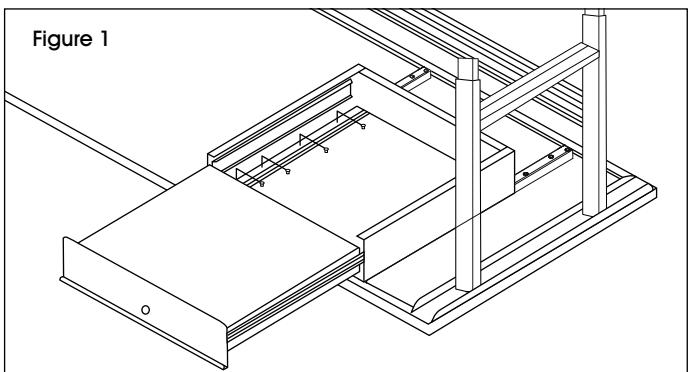
3. Close the drawer and turn the packing table right side up. Cycle the drawer in and out a few times to check operation.
