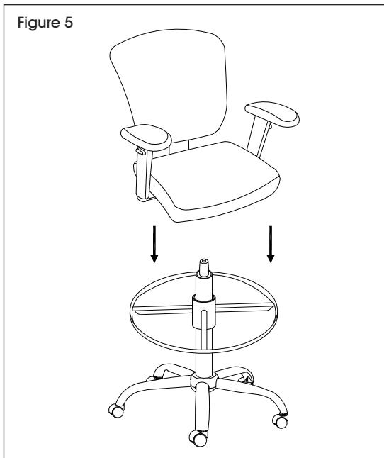
5. Slowly lower stool assembly onto the gas lift. Press down on seat cushion to secure. (See Figure 5)
