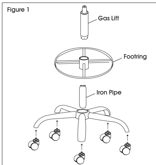
1. Insert casters or glides into legs of five-star base. Turn base upright. Insert iron pipe into center of base. Set footring on top of iron pipe and then insert gas lift into center of footring. (See Figure 1)
