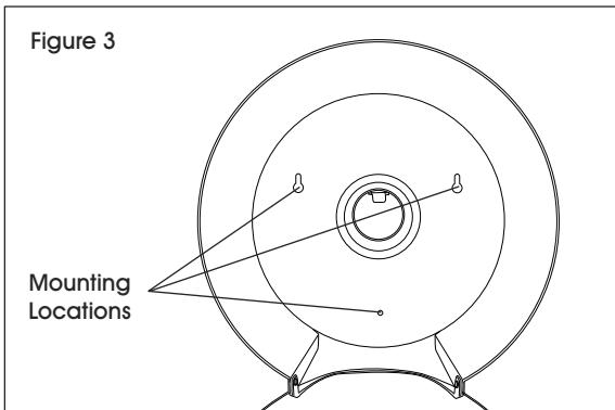
4. Drill into wall at three marked locations with appropriate size drill bit. (See Figure 4) Insert wall anchors if necessary.
