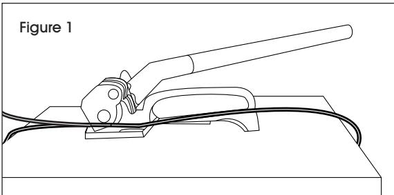
3. Squeeze handle toward base and insert strapping under the gripper.
