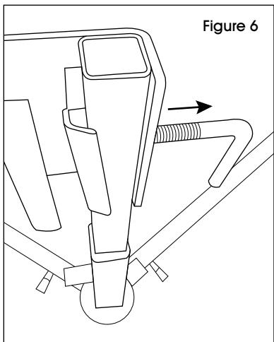
8. Tighten screw until the locking mechanism secures the sign in place. (See Figure 8)
