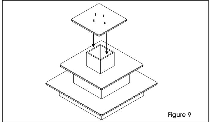
8. Set the top box stand on top of the four long camlock pins on the middle table. Insert screwdriver into the remaining four embedded camlocks at the bottom and turn clockwise to secure box stand to the table. (See Figure 8)
