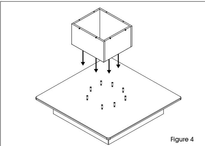
5. Embed eight short camlock pins to the bottom of the middle table, and set on top of the bottom box stand. Turn the eight outside screws clockwise to secure the middle table. (See Figure 5)
