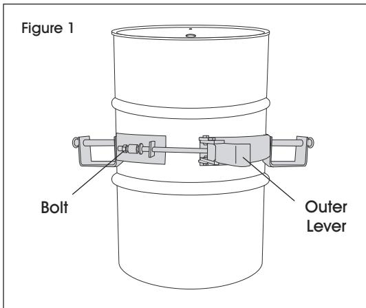
3. Using bolt, firmly tighten tilt ring around the drum, locking it into place. (See Figure 3)
