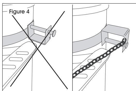
5. Attach safety chains from tilt ring to forklift to prevent tilt ring from sliding off forks when in use.
