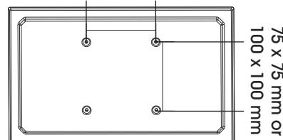
1. Easy-adjust monitor mount includes a built-in counterweight system for free-range motion. Arm in mount may need to be adjusted to allow monitor to stop at desired position. Attach monitor to plate. (See Figure 37)
