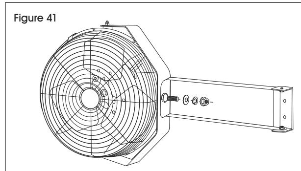
3. Align fan assembly with uprights at desired height.
