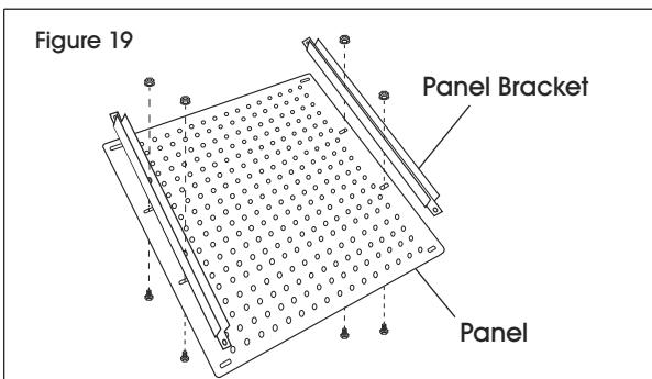
4. Repeat for additional panels. The 48" workstation holds up to 2 panels, 60" and 72" workstations hold up to 3 panels, and the 96" workstation holds up to 4 panels.
