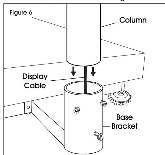
wrench and with the socket cap bolt using a 4.5 mm Allen wrench, but do not tighten.
