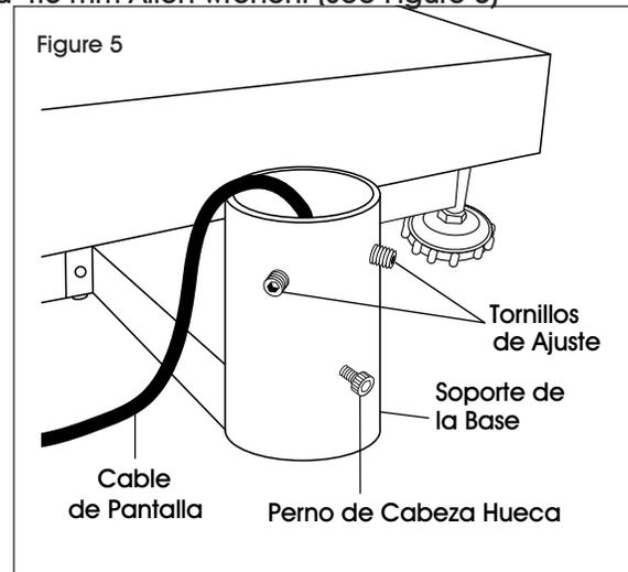
3. Insert column into base bracket. Make sure column rests on the bottom of the base bracket. (See Figure 6) Pull display cable all the way through the column so no slack is under the platform.
