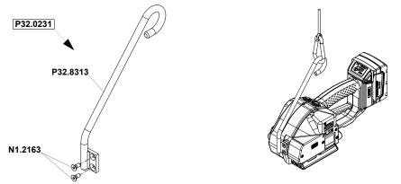
With the swivel mounted suspension bracket the package can be strapped in various working positions. The complete suspension bracket can be ordered under item number P32.0223.
