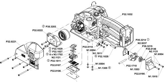
Insert part P32.8198 only for strap thickness 0.65-1.05mm
