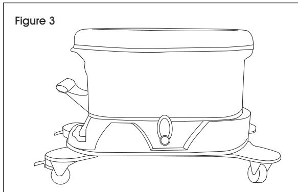
4. To move dolly, unlock wheels by pressing up on wheel locks. (See Figure 4)
