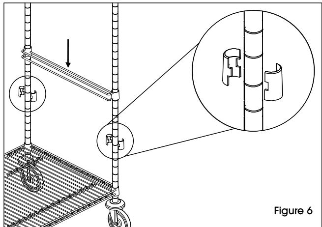
5. Repeat this process with the remaining box slides with 6" between each set of shelf supports.
