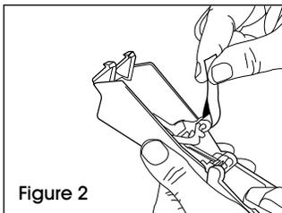
2. Insert folded backing paper between ink roller and carrier. Pull to snap old ink roller free. (See Figure 2)
