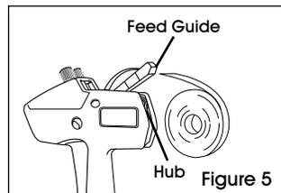
3. Place the label roll between the hubs and click into place. (See Figure 5)
