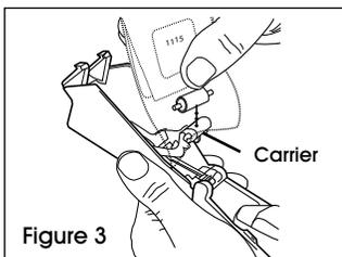
3. Cut off end of ink roller package. Using package to protect fingers, slide carrier into package and snap new ink roller into place. (See Figure 3)
