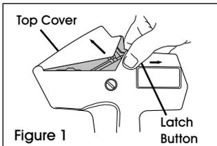
1. Push the two latch buttons in toward label roll and swing top cover away from print head. (See Figure 1)
