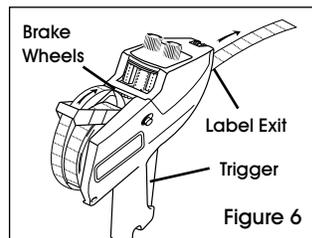
5. Squeeze and hold the trigger while feeding the label strip into the slot below the brake wheels until about 6" come out of the front. (See Figure 6)
