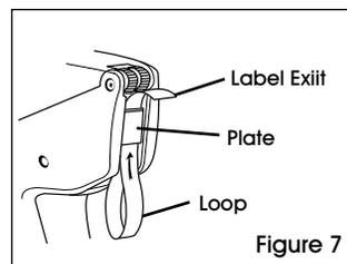
6. Feed label strip under the plate and pull through until loop is removed. (See Figure 7)
