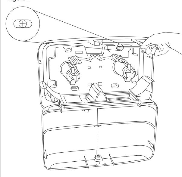
4. Ensure the dispenser is level by looking at the level bar on the inside of the dispenser. If level, screw in last three screws. (See Figure 8)
