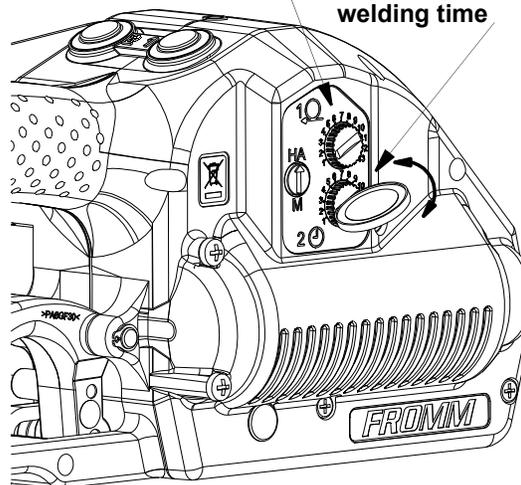
The adjustment knobs can be easily turned with a coin.
