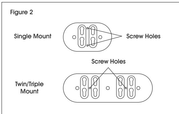
2. Screw the wall plate to the wall using previously marked screw holes.
